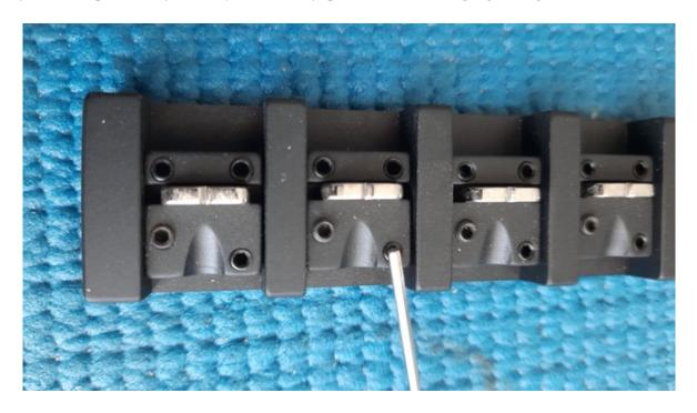
4. This screw hidden under the string releases/locks the saddle proper and allows it to slide L/R inside its channel to set custom string spacing. I don't advise increasing/decreasing it by more that 0.5mm as the added distance compounds pushing the outer saddles beyond the maximum channel length.
